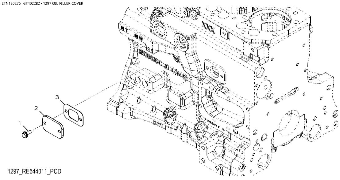
John Deere > Turf And Utility >TRACTOR >6090RC - TRACTOR >6090RC Tractor (Europe Edition, Engine SN: 4045RXXXXXX)(Interim Tier 4) >20 ENGINE 4045HL490-DD22206-DD22370-ETN98548-ETN120276 >ST402282 - 1297 OIL FILLER COVER
