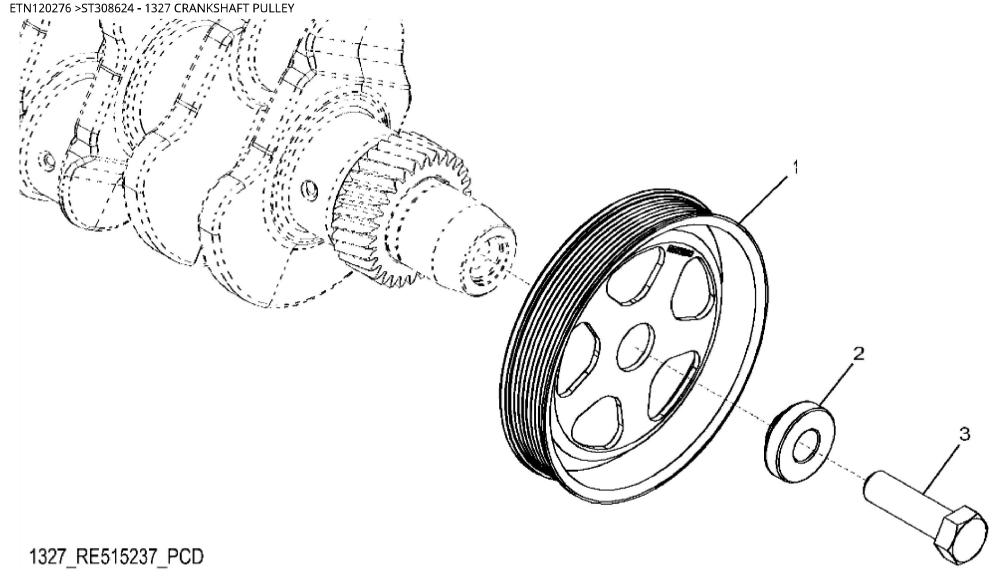
John Deere > Turf And Utility >TRACTOR >6090RC - TRACTOR >6090RC Tractor (Europe Edition, Engine SN: 4045RXXXXXXX)(Interim Tier 4) >20 ENGINE 4045HL490-DD22206-DD22370-ETN98548-ETN120276 >ST308624 - 1327 CRANKSHAFT PULLEY
