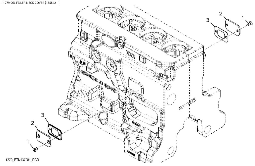
John Deere > Turf And Utility > TRACTOR > 6150M - TRACTOR > 6150M Tractor (Europe Edition, Engine SN: 6068GXXXXXXX)(Tier 2)(S.N. -860503) > 20 ENGINE 6068HL286-DD22382-ETN108063 > ST852078 - 1279 OIL FILLER NECK COVER (155842 - )
