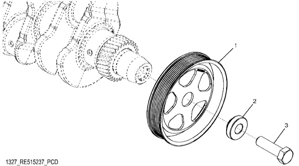
John Deere > Turf And Utility >TRACTOR >6130R - TRACTOR >6130R Tractor (North America Edition, Engine SN: 4045UXXXXXX)(Final Tier 4) >E1 ENGINE 4045HL500-DD22292-ETN122284-ETN122286-ETN131686 >E100 ENGINE 4045HL500-DD22292-ETN122286-ETN131686 4045HL500 >ST308624 - 1327 CRANKSHAFT PULLEY
