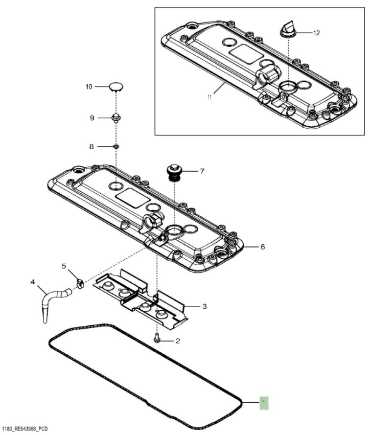
John Deere > Turf And Utility >TRACTOR >6130R - TRACTOR >6130R Tractor (North America Edition, Engine SN: 4045UXXXXXX)(Final Tier 4) >E1 ENGINE 4045HL500-DD22292-ETN122284-ETN122286-ETN131686 >E100 ENGINE 4045HL500-DD22292-ETN122286-ETN131686 4045HL500 >ST400926 - 1183 ROCKER ARM COVER
