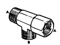
816/50005 1/2 in BSP (A) x 1/2 in BSP (B) 816/60096 3/4 in BSP (A) x 3/4 in BSP (B) 816/00018 1 in BSP (A) x 1 in BSP (B)
