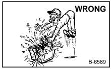
Lead-acid batteries produce flammable and explosive gases. Keep arcs, sparks, flames and lighted tobacco away from batteries.
