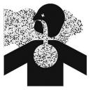
Cutting or drilling concrete containing sand or rock containing quartz may result in exposure to silica dust.
