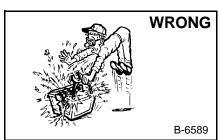
Lead-acid batteries produce flammable and explosive gases.
