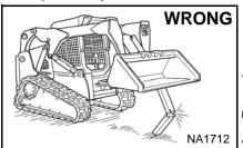
Never work on loader with lift of arms up unless lift arms are held by an approved lift arm support device. Replace if damaged.
