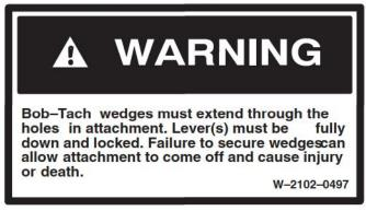
The spring loaded wedge (Item 1) [A] must contact the lower edge of the hole in the attachment (Item 1) [B] and [C].
