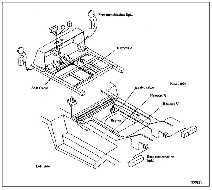
For the components to which harnesses A, B and C are connected, see the pages which follows.
