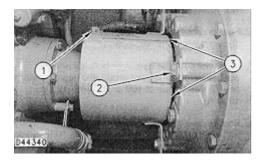
**2.** Remove bolts (1), the washers, bolts (2) and the washers from two guards (3). Remove two guard (3) from the front of the transmission.
