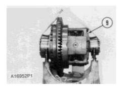
**8.** Fasten a hoist and a strap to the differential (9) as shown. Lift the differential and remove it from the carrier. Weight is 240 lb. (109 kg).
