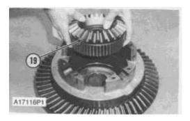
17. Remove gear (19) from the housing.
