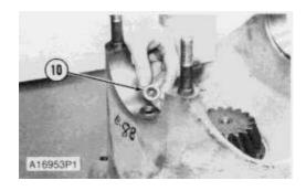
**9.** Remove the ring and seal (10) from the carrier.
