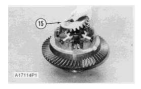
**13.** Remove gear (15) from the spinder gears.
