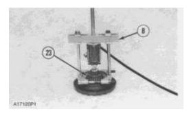
21. Remove bearing (23) from the piston housing with tooling (B).
