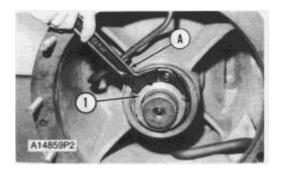
1. Bend the lock away from nut (1) and loosen nut (1) with tool (A).
