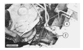
3. Install the fourteen bolts (2) that hold the swing drive to the frame. Tighten the fourteen bolts to a torque of  $880 \pm 80$  lb.ft. (1190  $\pm$  110 N·m) with tool (A).
