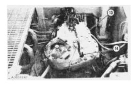
**10.** Install three 1/2" - 13 NC forged eyebolts (14). Fasten a hoist and remove the swing drive (13). Weight of swing drive is 1650 lb. (743 kg).
