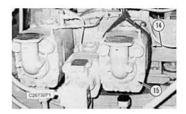
**5.** Fasten a hoist to front pump (15). Remove two bolts (14) holding the front pump to the pump drive housing and remove front pump (15). Weight of the front piston pump is 935 kg (425 lb).
