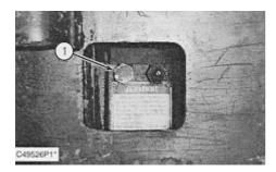
**2.** Release the tension on the track. Loosen relief valve (1) only one turn. If the track does not loosen after opening the relief valve, move the machine forward and backward until the tension is released.
