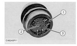
**2.** Remove plug (2), and drain the oil from the carrier roller in a suitable container for disposal. The capacity of the track carrier roller is  $120 \pm 5 \text{ ml} (4.08 \pm 0.17 \text{ oz})$ .
