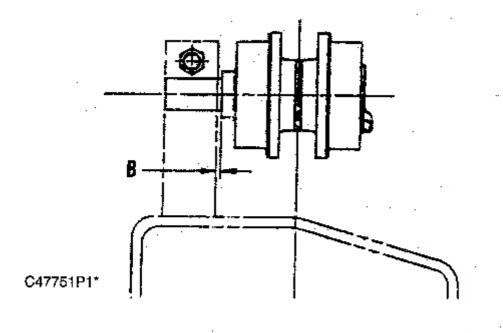
6. Put the track carrier roller in position in the mounting bracket. Adjust the carrier roller until distance (B), the distance between the outside face of the mounting bracket and the carrier roller is  $7.0 \pm 0.5 \text{ mm} (.28 \pm .02 \text{ in}).$
