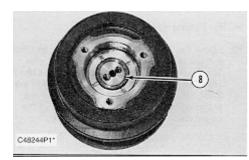
6. Carefully remove shaft assembly (8) from the track carrier roller.
