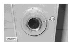
11. Remove two lip seals (15) from the stick at the stick-to-bucket linkage pin joint.
