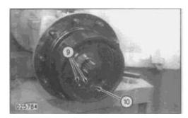
7. Loosen both hex head screws (9) and remove lock plate (10).
