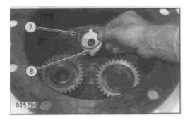
6. Remove snap ring (7) and remove thrust washer (8).
