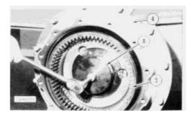
**2.** Use tool (A) to remove nut from spindle. Install tooling (B) on wheel assembly (4) and remove gear assembly (5) from wheel assembly.
