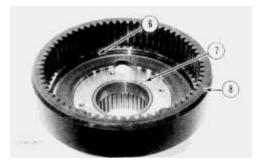
**3.** Remove retaining ring (6) from hub assembly (7) and remove ring gear (8).
