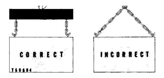
When it is necessary to remove a component on an angle, remember that the capacity of an eyebolt diminishes as the angle between the supporting members and the object becomes less than 90°. Eyebolts and brackets should never be bent and should only have stress in tension. A length of pipe and a washer can be used, as shown, to help relieve these stresses on eyebolts.
