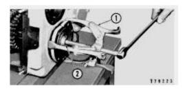
EXAMPLE OF TOOL INSTALLATION 1. Puller. 2. Step plate.
