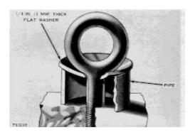
Some removals require the use of lifting fixtures to obtain proper balance and to provide safe handling.
