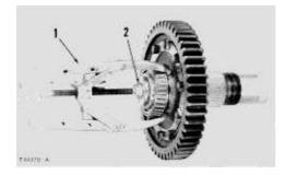
EXAMPLE OF TOOL INSTALLATION 1. Puller. 2. Step plate.
