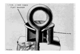
Some removals require the use of lifting fixtures to obtain proper balance and to provide safe handling.
