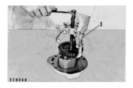
EXAMPLE OF TOOL INSTALLATION 1. Puller.
