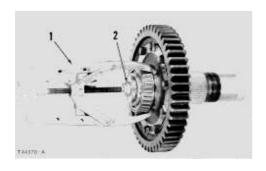
EXAMPLE OF TOOL INSTALLATION 1. Puller. 2. Step plate.
