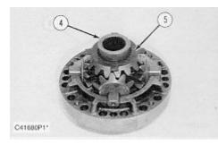
6. Install bevel gear (4) and thrust washer (5) in the case assembly.
