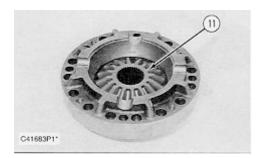
2. Install bevel gear (11) in the case assembly.
