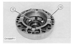
1. Install thrust washer (12) in case assembly (13).
