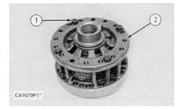
7. Put case assembly (2) in position, and install four bolts (1) and the washers that hold it.
