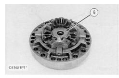
**3.** Remove spider and gear assembly (6).
