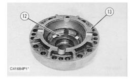
7. Remove thrust washer (12) from case assembly (13).
