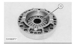
6. Remove bevel gear (11) from the case assembly.
