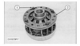
1. Remove four bolts (1) and the washers that hold case assembly (2). Remove the case assembly.
