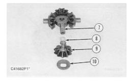
**3.** Assemble the spider and gear assembly. Install sleeve bearing (8), bevel pinion (9) and thrust washer (10) on spider (7).
