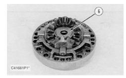
5. Install spider and gear assembly (6) in the case assembly.
