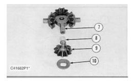
**4.** Disassemble the spider and gear assembly. Remove thrust washer (10), bevel pinion (9) and sleeve bearing (8) from spider (7).
