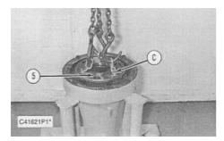
**5.** Fasten Tool (C) and a hoist to planetary carrier assembly (5) as shown. Remove the planetary carrier assembly from the axle shaft housing. The weight of the planetary carrier assembly is approximately 80 kg (175 lb).
