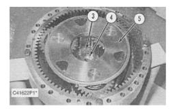
**3.** Remove the bottom half of the axle housing group from Tool (G). Install axle shaft assembly on Tool (G) with planetary carrier assembly (5) facing up as shown.
