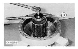
**7.** Fasten the rim flange of the axle shaft to Tool (G) with suitable size bolts as shown in Photo C42124P1. Installation of the bolt will prevent the axle shaft from turning when bearing nut (12) is removed. Use Tooling (D) to remove bearing nut (12) from the axle shaft.
