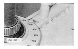
The axle shaft housing has been removed from the axle shaft for better photo illustration of mounting the axle shaft to Tool (G).
