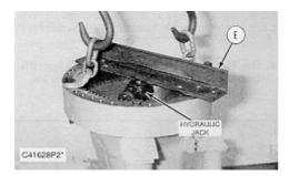
**NOTE:** The bearing cone which is located under bearing nut (12) will be removed at the same time that the axle shaft housing is being removed from the axle shaft.
