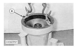
**8.** Fasten Tooling (A) and a hoist to the axle shaft housing as shown. Put slight lifting tension on the axle shaft housing.
