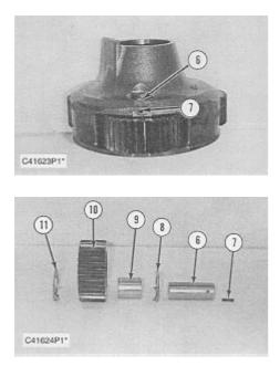
6. Disassemble planetary carrier assembly (5) as follows:
