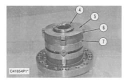
**5.** Install pressure ring (7), two inner discs (6), two outer discs (5) and thrust washer (4).
