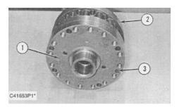
**6.** Install differential housing (2). Install two socket bolts (3). Tighten socket head bolts (3) to a torque of  $54 \pm 10 \text{ N} \cdot \text{m}$  ( $40 \pm 7 \text{ lb ft}$ ).
