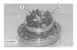
**3.** Install bevel gears (10) on pinion shafts (9). Install the bevel gears and pinion shafts on the pressure ring.
