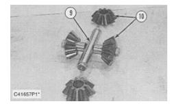
**4.** Remove four bevel pinions (10) and two pinion shafts (9).
