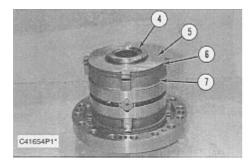
2. Remove thrust washer (4), two outer discs (5), two inner discs (6) and pressure ring (7).
