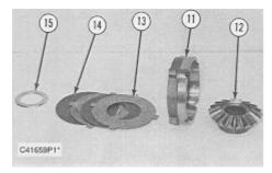
**5.** Remove bevel gear (12), pressure ring (11), two outer discs (13), two inner discs (14) and thrust washer (15).
