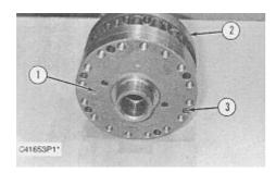
**1.** Remove two socket head bolts (3). Turn the differential up on differential housing cover (1), and remove differential housing (2).
