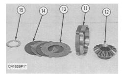
**2.** Install thrust washer (15), two inner discs (14), two outer discs (13), ring (11) and bevel gear (12) on differential housing cover (1).
