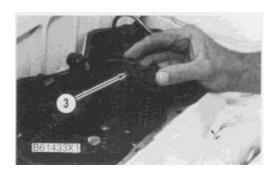
**6.** Put bridges (3) into position on the lifters as shown.
