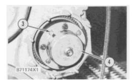
2. Remove bolts (3) and automatic timing advance (4) from the engine.
