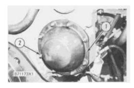
1. Remove nuts (2), cover (1) and the gasket from the timing gear cover.
