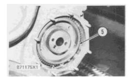
**3.** Remove gear (5) from the timing gears.
