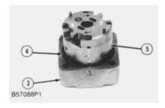
**4.** Remove O-ring seal (4) and cartridge (5).
