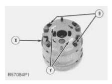
**NOTE:** Make a note of the directions of the arrows at locations (X) and (Y) and the location of bolts (9) for correct assembly purposes. The arrows indicate the direction of rotation of the hydraulic oil pump. Bolts (9) are installed in the holes next to the arrows that show the direction of pump rotation.
