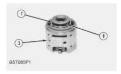
**6.** Remove back-up ring (7) and O-ring seal (8).
