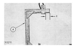
5. Adjust the bracket on Tooling (A) until dimension (X) is 225 mm (9 in).
