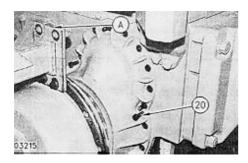
10. Turn pusher bolts (20) and remove the final drive assembly. The final drive assembly weight is 322 Kg (710 lb).
