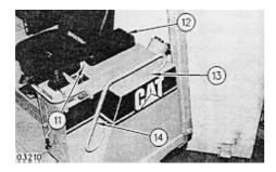
4. Remove two bolts (11) and cushion assembly (12). Remove two bolts (13) and handhold (14).
