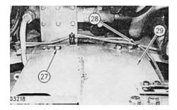
13. Cut strap (28) and remove eight bolts (27), washers and plate (29).
