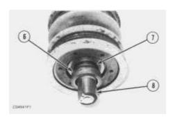
**6.** Remove seal ring (6) and toric stabilizer (7) from shaft (8).
