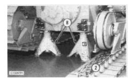
**3.** Raise the rear of the tractor until track guides (2) are above the track links. Put tooling (B) in position under the tractor as shown. Lower the tractor onto tooling (B).
