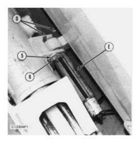
**6.** Remove bolt (6) from the equalizer bar pin and the track roller frame. Install tooling (D) on each side of the pin, between the equalizer bar and the track roller frame as shown.
