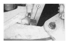
**1.** Put tooling (A), bar stock, in position between the equalizer bar and main frame on the same side that the track roller frame is to be removed from. This will keep the equalizer bar in its original position when the track roller frame is removed.
