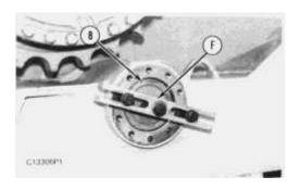
9. Use tooling (F) and remove retainer (8) from the track roller frame.
