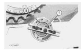
**9.** Use tooling (F) and remove retainer (8) from the track roller frame.
