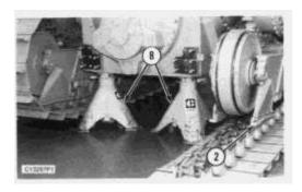
**3.** Raise the rear of the tractor until track guides (2) are above the track links. Put tooling (B) in position under the tractor as shown. Lower the tractor onto tooling (B).
