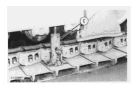
**5.** Put tooling (C) in position under the roller frame as shown. Use tooling (C) to put pressure on the track roller frame.
