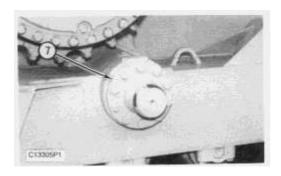
**8.** Remove the bolts and push arm trunnion (7) from the track roller frame.
