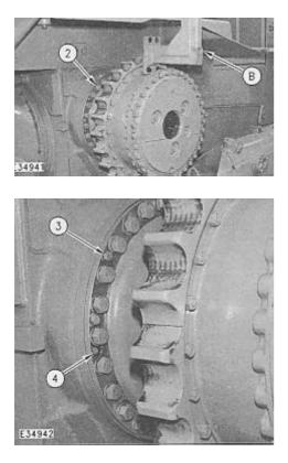
**5.** Remove two of the bolts from the sprocket segments. Fasten a hoist and install Tooling (B) on the final drive.
