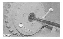
7. Install Tool (A) on the outer axle and install the axle in the final drive.
