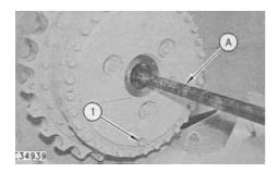
**1.** Turn the final drive until drain plug (1) is on the bottom as shown. Remove drain plug (1) and drain approximately 13.2 liters (3.4 U.S. gal.) of oil from the final drive.
