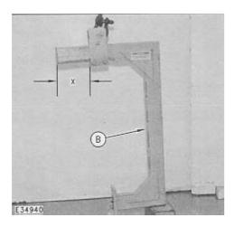
**4.** Adjust the top bracket on Tooling (B) so that dimension (X) is 213 mm (8.4 in). The lower mounting bracket must be installed with the spacers outward as shown.
