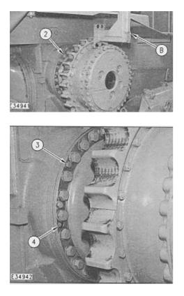
**3.** Fasten a hoist and install Tooling (B) on the final drive. Adjust Tooling (B) if necessary to put the final drive in a level position.
