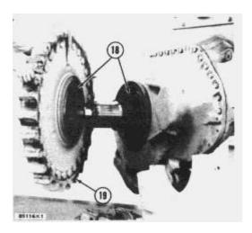
12. Fasten a hoist to the sprocket (19) and remove it. Weight is 700 lb. (318 kg).
