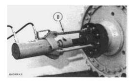
**8.** Loosen the support and bearing cones from the sprocket hub with tooling (D).
