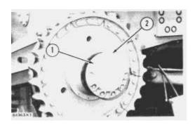
**2.** Remove bolts (1) that hold the cap to the support. Install two 1/2"-13NC forcing screws into the cap. Remove cap (2) and its shims.
