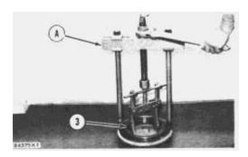
**3.** Remove the bearing race (3) from the cap with tooling (A).
