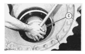
7. Remove nut (13) and spacer with tool (C).
