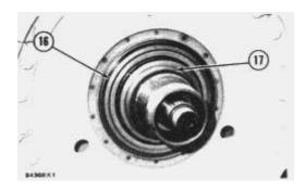
**10.** Remove the Duo-Cone seal (16) and spacer (17) from the sprocket. Keep the Duo-Cone seals for the sprocket and support together to prevent mixing at assembly.
