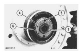
**4.** Remove bolts (5) and lock (6). Remove nut (7) from the shaft. Remove bearing cone (4) from bearing cage.
