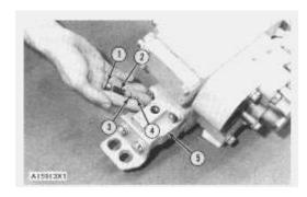
1. Remove detent plugs (1), springs (2), seats (3) and balls (4).
