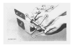
14. Remove plug (31), spring (30) and valve (29) from body of valve.
