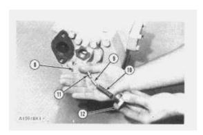
**5.** Remove two plugs, (8) and (12) from the valve body. Remove shims (in the plugs), pistons (9), springs (10) and valves (11) from the valve body.
