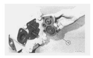
**6.** Remove four bolts from cover (13) and remove from valve body.
