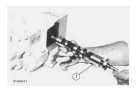
**4.** Carefully remove spool valve (7) from valve body.
