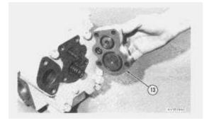
6. Remove four bolts from cover (13) and remove from valve body.
