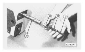
12. Remove springs (22) and (23), sleeve (21) and spool (24) from valve body.
