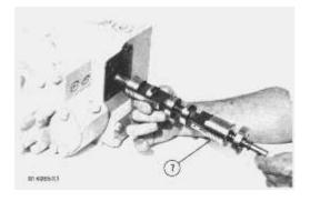
**4.** Carefully remove spool valve (7) from valve body.
