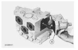
3. Remove four bolts from control lever housing (6) and remove housing from valve body.
