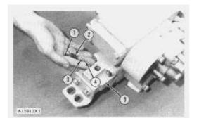
1. Remove detent plugs (1), springs (2), seats (3) and balls (4).
