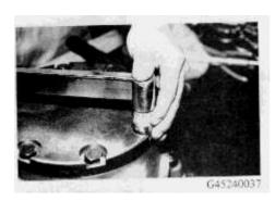
**3.** Remove two hexagon bolts positioned symmetrically with a socket and a torque wrench.
