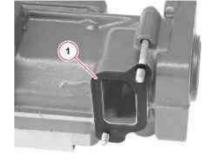
• Fit the charge air duct.
