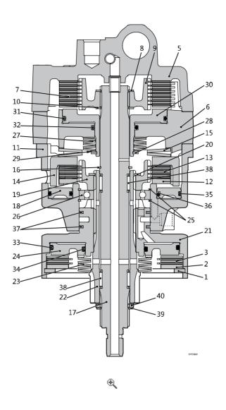
Fig. Clutches assembly
