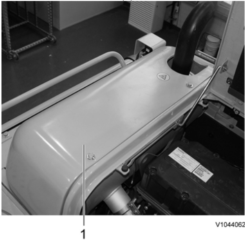
Figure 3 Removal, silencer hood
