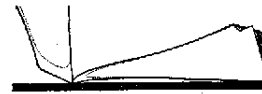
Figure 10—Unbroken Lines in Overhead and Side Views of Share Above Show Correct Shape for Penetration. Dotted Lines Show How Worn Point Looks Before Sharpening
