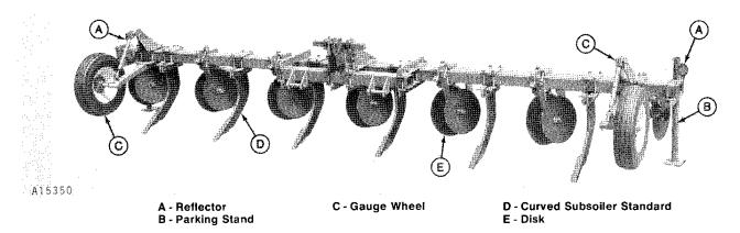
John Deere 6 Row - 990 Subsoiler Bedder Single Bar with Staggered Disks (Gauge Wheel and Support Stand-Attachments)
