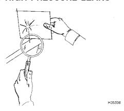
Escaping fluid under pressure can have sufficient force to penetrate the skin, causing serious injury. Before disconnecting lines, be sure to relieve pressure. Before applying pressure, be sure connections are tight and lines, pipes and hoses are not damaged. Use a piece of cardboard or wood, rather than hands, to search for leaks.
