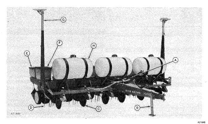
A-Liquid Fertilizer Metering Pump
