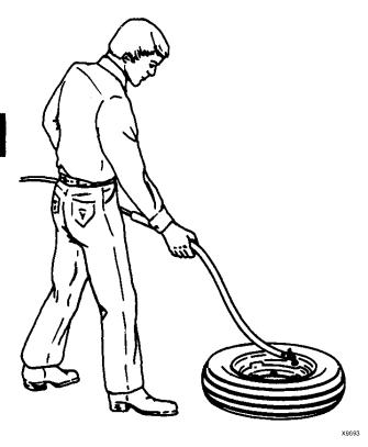
Failure to follow proper procedures when mounting a tire on a wheel or rim can produce an explosion which may result in serious injury or death. Do not attempt to mount a tire unless you have the proper equipment and experience to perform the job. Have it done by your John Deere dealer or a qualified tire repair service.
