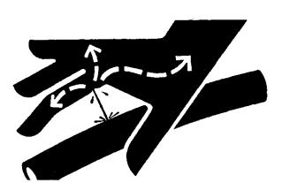
Escaping fluid under pressure can penetrate the skin causing serious injury. Relieve pressure before disconnecting hydraulic or other lines. Tighten all connections before applying pressure. Keep hands and body away from pinholes and nozzles which eject fluids under high pressure. Use a piece of cardboard or paper to search for leaks. Do not use your hand.
