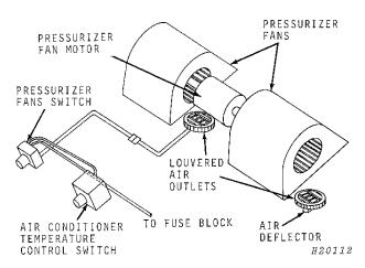
The pressurizer system consists of two rotating cage-type fans, an electric motor, two louvered air outlets, an air deflector (snapped into one of the air outlets) and a control switch.
