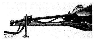
Install hydraulic cylinder as shown. Attach hoses to cylinder and route as shown, being careful not to crush or pinch hoses.
