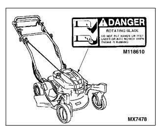
Do not put hands or feet under or into mower when engine is running.
