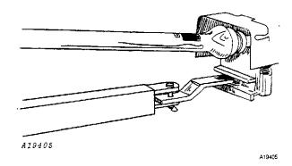
Keep guards and shields in place at all times while operating the combine. Alwasy disengage tractor PTO and shut off engine before removing guards or shields.
