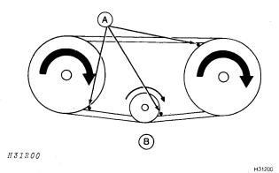
Keep hands, feet, and clothing away from power-driven parts. Be particularly careful of pinch points on belt and chain drives.
