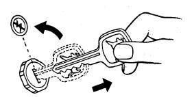
Before leaving the combine unattended, turn off engine and remove keys. Support the row-crop head with the hydraulic cylinder safety stop or lower it to the ground. Place the gearshift lever in neutral and engage the parking brake. Lock cab doors on 6620, SideHill 6620, 7720 and 8820 Combines.
