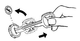
Before leaving the combine unattended, turn off engine and remove keys, support the platform with either the hydraulic cylinder safety stop, or lower it to the ground. The gearshift lever must be in neutral and the parking brake engaged. Lock cab doors.
