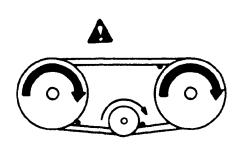
Keep guards and shields in place at all times while operating the combine. Always disengage separator and shut off engine before removing guards or shields.
