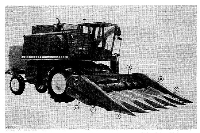
A—Cross Auger B—Inner Gatherer Sheet C—Inner Gatherer Point D—Row Unit Drive Shield
