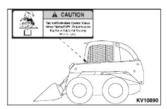
Read and Understand Operator Manual Before Raising ROPS. Failure to do so May Cause Cab to Fall Causing Serious Injury.
