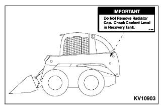
Do Not Remove Radiator Cap. Check Coolant Level in Recovery Tank.
