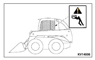
Remove the rear window to provide an exit in an emergency when the front exit is blocked.
