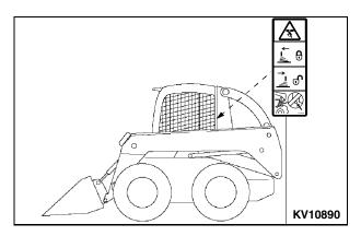
If you must leave boom raised when exiting, be sure boom locks are in the LOCKED position and the boom is resting on the locks.
