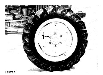
1 After having adjusted front wheel tread tighten front wheel attaching cap screw ball nuts to 320 Nm (32 mkp - 240 ft-lb) torque.
